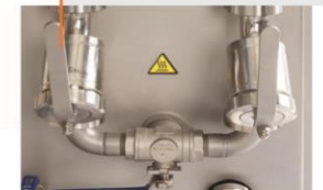
Double glaze filter to prevent nozzle blockage
