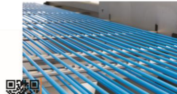
Conveyor with poly cords (or wire mesh) and adjustable speed
