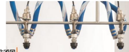
Spray bridge with adjustable spray guns
